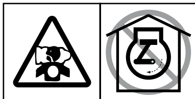
The Engine emits toxic Carbon Monoxide. Do not run the Engine in an enclosed area.
